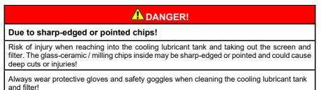
The cooling lubricant tank must be emptied and cleaned every two weeks. Always dispose of cooling lubricant residues in accordance with the legal provisions and local regulations!
